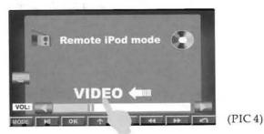
Touch "VIDEO" on the main menu and the unit will switch to " ipod "operation mode, while, control the "ipod" player, and select the video file you want to play, while the video picture will transfer to the unit screen. During the unit playing the video, "ipod" player must set as Video mode, if not the unit only with audio but not video.
